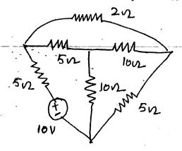
5. (a) For the network shown, determine the current i(t) when switch is closed at t = 0 10 with zero initial conditions.
