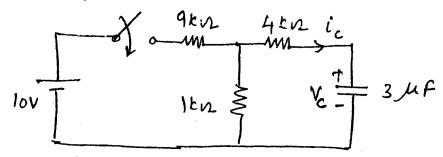
(b) Calculate the twig voltages using KCL equation for the network shown.
