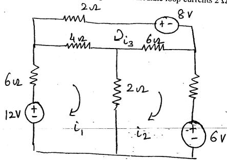
3. (a) In the network shown what will be the  $R_L$  to get maximum power delivered to it ? 10 What is the value of this power ? 5V
