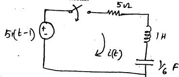
(b) Find impulse response of voltage across the capacitor in the network shown. Also 10 determine response V<sub>c</sub>(t) for step input.
