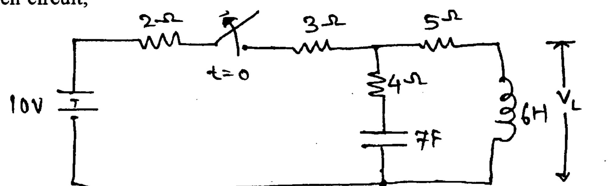
switch 's' is opened at t=o. Switch 's' was on for long time.
