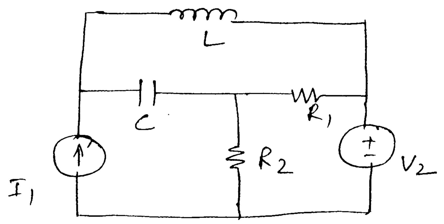
(b) Determine  $i_1, i_2, \frac{di_1}{dt}, \frac{d^2i_1}{dt^2}, \frac{d^2i_2}{dt^2}$  at  $t = 0^+$  in the circuit shown :—
