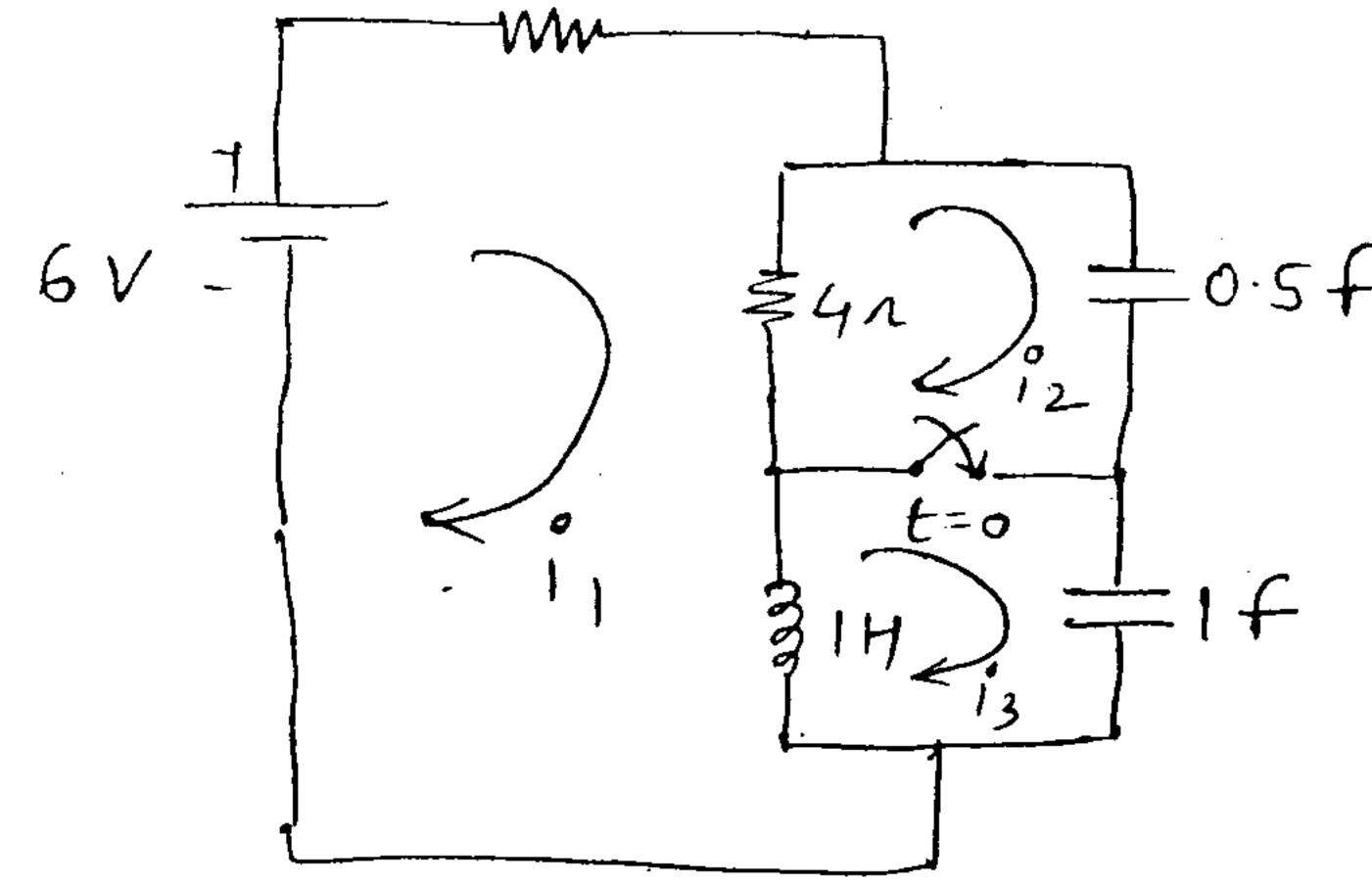
(b) Find i(t) for the circuit given using Classical method:-
