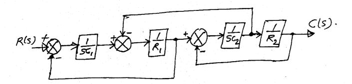
(a) Obtain the overall transfer function of a control system shown by following Signal 10 3.
