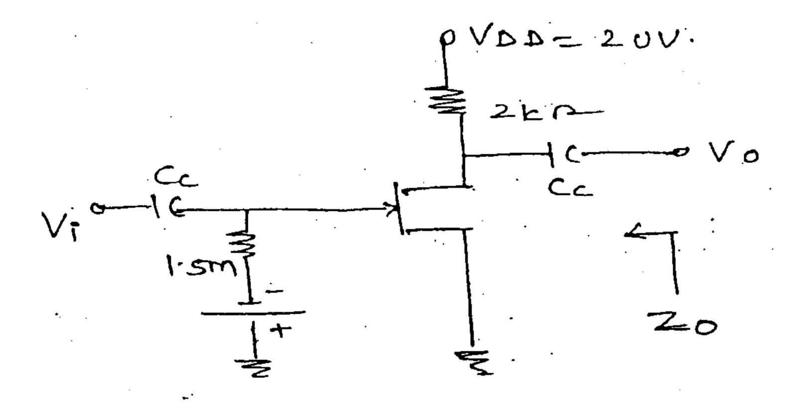
(b) An Amplifier circuit shown in Fig. Determine the co-ordinates of the operating point Q and thermal stability
