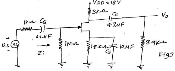
For JFET  $I_{DSS} = 6 \text{ mA}$ ,  $V_p = -6 \text{ V}$ ,  $r_{dl} = \infty$ ,  $C_{gd} = 4 \text{ pF}$ ,  $C_{gs} = 6 \text{ pF}$ ,  $C_{ds} = 1 \text{ pF}$  and  $C_{wi} = 3pF$ ,  $C_{wo} = 5 pF$ .
