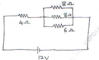
(b) Find the Thevenin's equivalent ckt for the below circuit-as seen from A-B.
