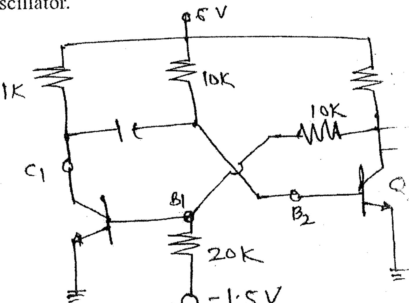
For the above circuit, compute voltage levels and sketch the waveform at  $B_1$ ,  $C_1$ ,  $B_2$  and  $C_2$  for permanant state and quasi Stable state. Use silicon transistors with  $r_{bb} = 100 \Omega$  and  $h_{FE} = 30$ .
