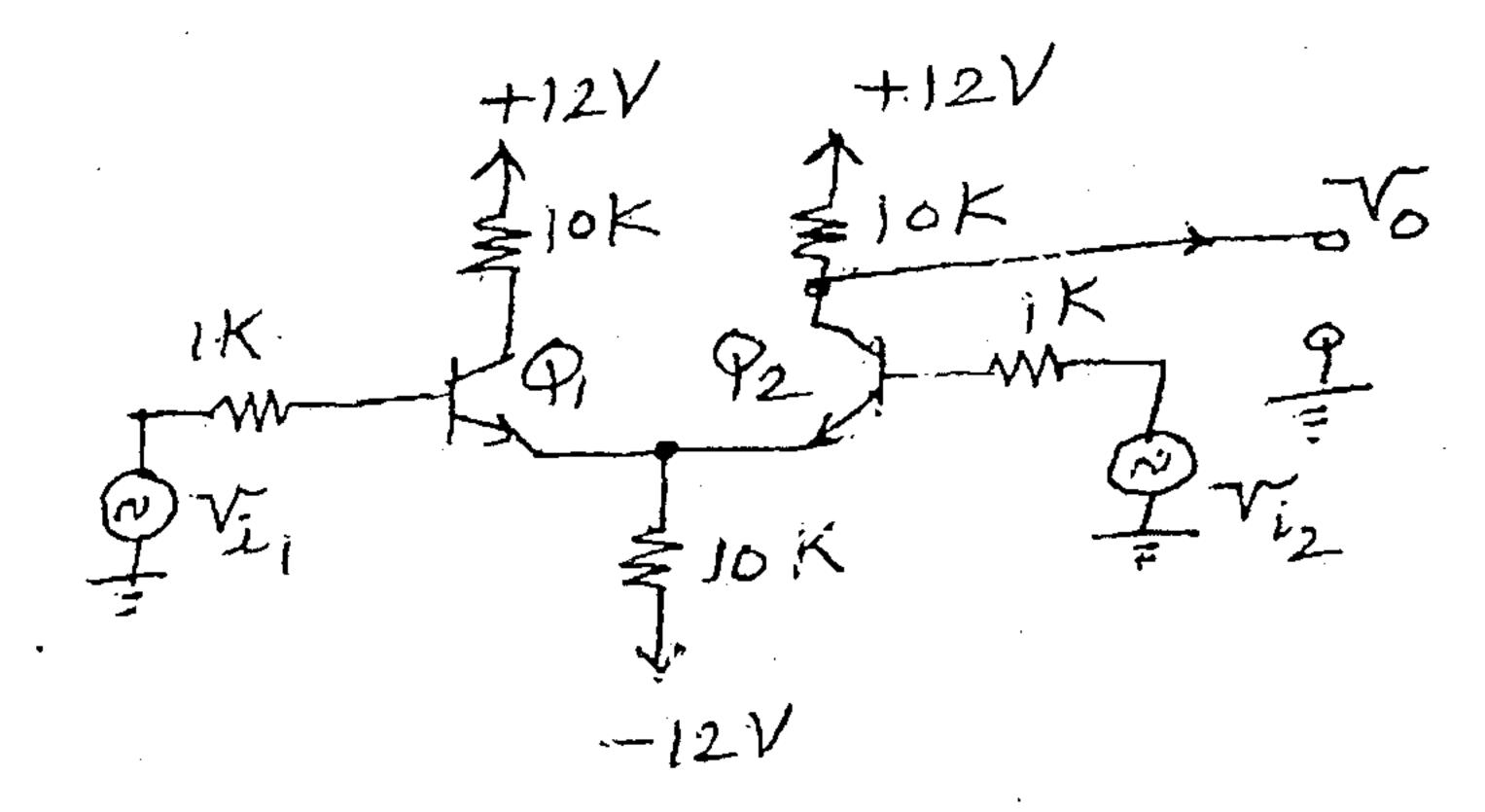
Transistors  $Q_1$  and  $Q_2$  are BC 147 A (refer to data table for transistor data) Neglect  $h_{oe} \& h_{re}$
