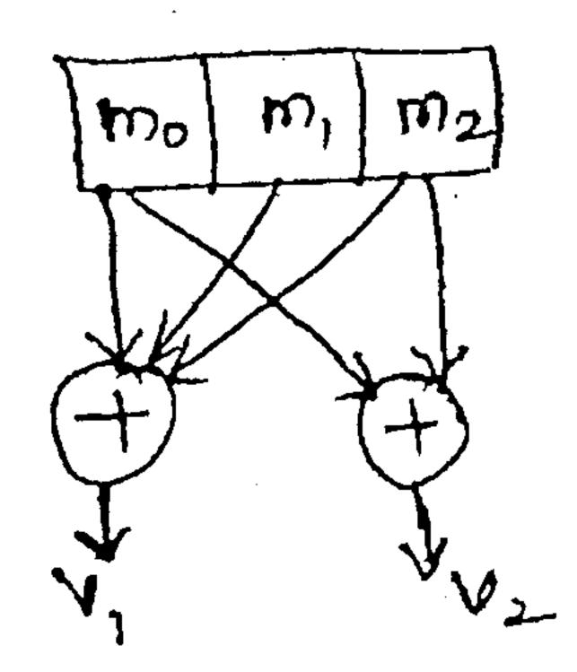
Obtain the convolution code for the input bit sequence 110011.
