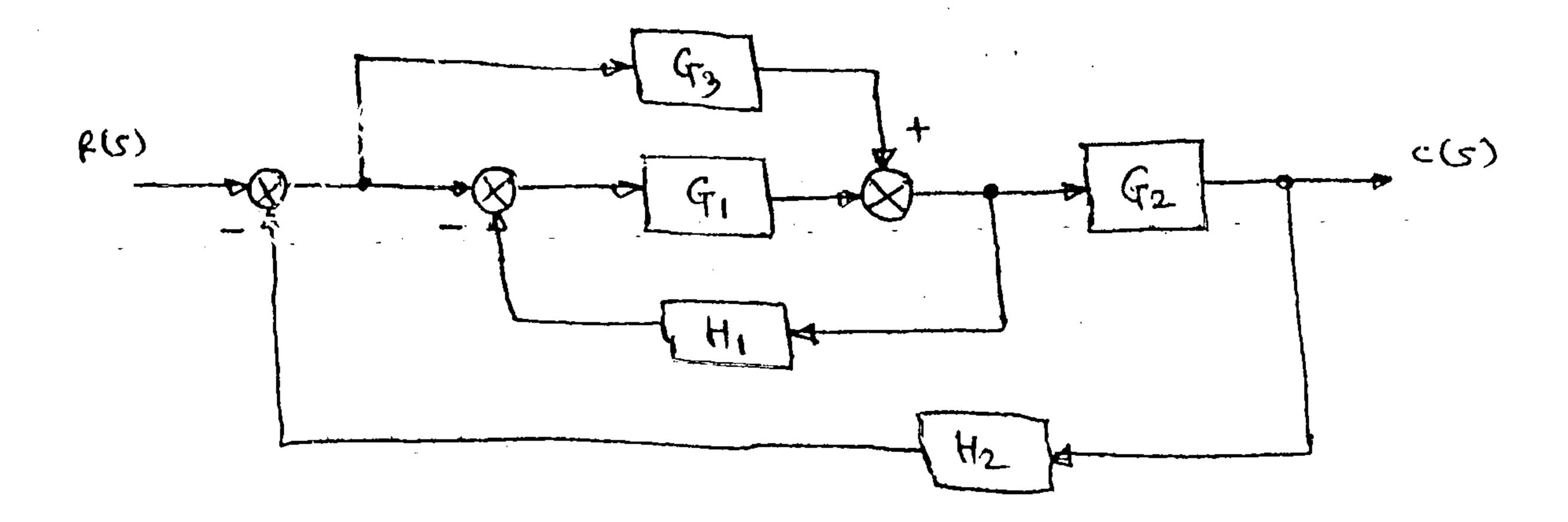
(b) Draw the corresponding signal flow graph of given block diagram and find  $\frac{C(s)}{R(s)}$ . 10
