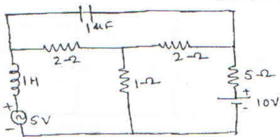
6. (a) Determine voltage across AB branch for the given network. 10
